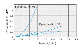
The flow resistence through the check valve, when the main valve is closed
