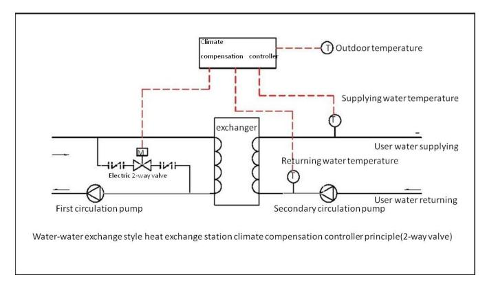
The above chart of the installation method is applied for limited place of remolding, the adjustment strength of the electric valve is smaller than the first two, The remote exchanger station can choose this installation.
