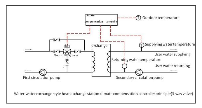
The above chart of the installation method, the adjustment of the electric valve won't cause the fluctuation of the water flow at one time, which is suitable for the heating company and the user' self-heating station.
