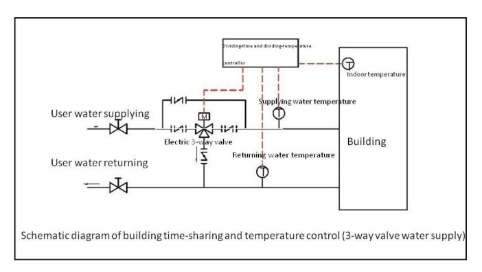
The installation method on the above is suitable for near-end buildings. The pressure of the near-end building is high, and the three-way split can be properly relieved.
