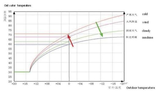
In above chart, four single curve is the supplying heat environment responding to different climate.
