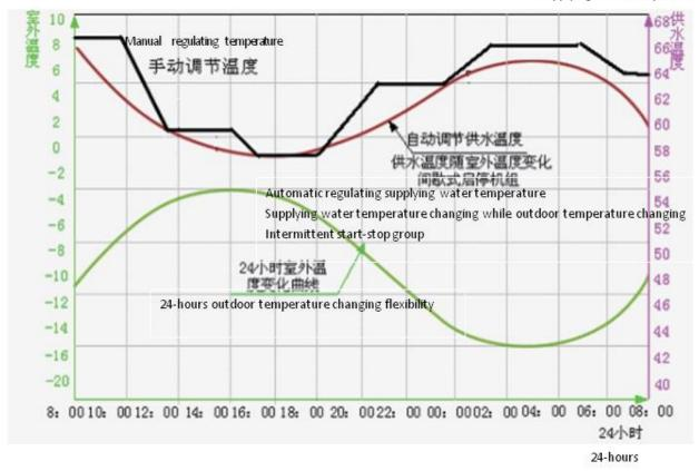
In above chart the black broken line is operating line of the outputting water temperature when operating the climate compensation by the manual regulating. The red line is the operating line of the outputting water temperature when the controller get the climate compensation done by itself. the green line is the 24 hours changing trend of the outdoor's temperature.
