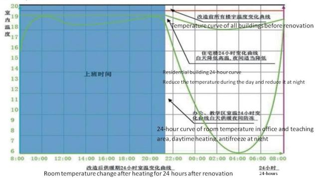
In the above figure, the red line is the uniform indoor temperature of all buildings before the renovation, which is basically smooth; the green shallow concave curve is the indoor temperature change of the residential area after the renovation: the green deep concave curve is the indoor temperature of the office building after the renovation Variety. The area of the concave portion shown in the figure is the energy saving after the dividing-time and dividing-temperature renovation.
