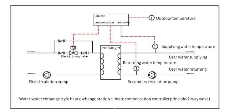
In the installation method on the above, the adjustment of the electric valve will cause a large fluctuation of the water flow at one time, which is suitable for the non-self-heating station, that is, the fluctuation of the flow can be automatically adjusted by the heat source of the heat company.
