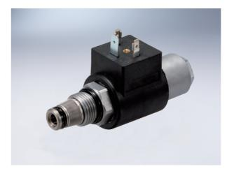
A solenoid-operated, 2-way, normally open, poppet-type, proportional, screw-in hydraulic cartridge valve for low-leakage load-holding applications, and for starting or stopping a load or a pump system.
