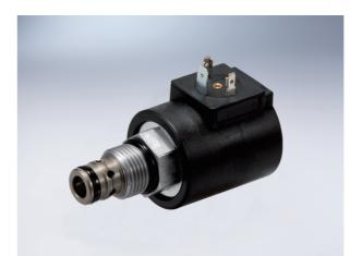
A screw-in, cartridge-style, pilot-operated, hydraulic pressure relief valve, which can be infinitely adjusted across a prescribed range using a variable electric input. Pressure output is inversely proportional to DC current input. This valve is intended for use as a pressure limiting device in demanding applications.
