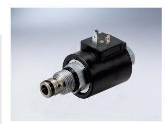
A screw-in, cartridge-style, pilot-operated, spool-type hydraulic relief valve, which can be infinitely adjusted across a prescribed range using a variable electric input. The regulated pressure is proportional to the input electrical current. This valve is intended for use as a pressure limiting device in demanding applications.
