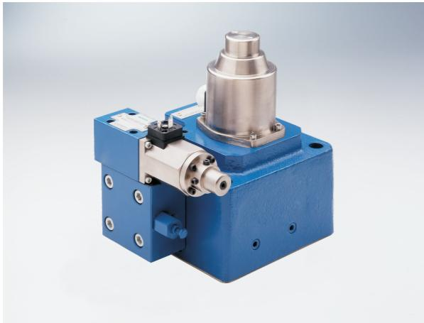
This proportional valve adopts two electrical loops to control pressure and flow of hydraulic system respectively. Using very small pressure drop to track load pressure and control the pump pressure, it is an energy-saving valve.
