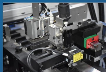
Press fit mechanism
