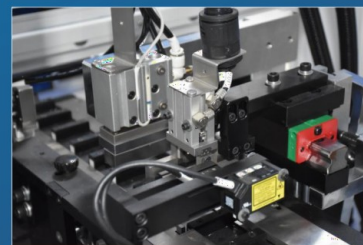
Press fit mechanism
