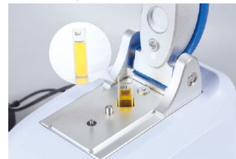
cuvette mode (Heating temperature 37 °C, speed 150-850 rpm)
