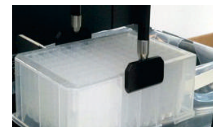
CO-RE gripper for plates transferring
