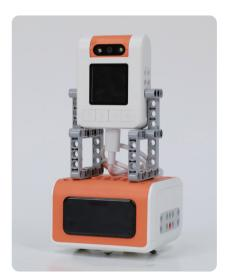
2 Turn on VinciBot and the screen lights up. Rotate the orange camera to check the preview image on the screen. For example, when the camera faces forward, the preview image is flipped.
