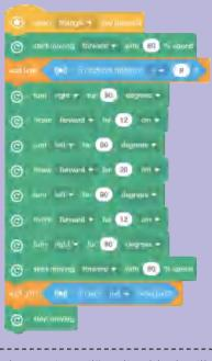
The "wait until" coding block will allow VinciBot to keep checking the conditions in this block; until the condition is met, the next instruction will not begin.
